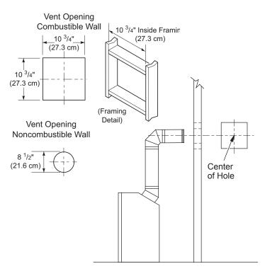
Figure 9 - Vent Opening Requirements
